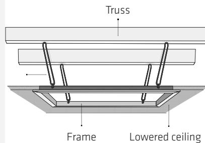
Hang the frame on the hooks in the enclosed wirers.
