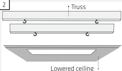
Measure and mount the four hooks in the trusses.
